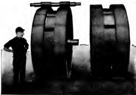
Reduction gears for the battleship "Idaho," cut in the shops of the De Laval Steam Turbine Company No. 1154.
